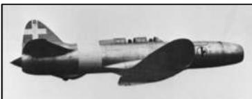
This is the Caproni Campini N1. It is an Italian aircraft that first flew in 1940. Pretty unique in that it had what was a rudimentary jet engine – which used a reciprocating engine to drive a compressor propeller which then fed compressed air to the "jet" part. Apparently the arrangement was so inefficient that the cockpit was always too hot for the crew – hence the aircraft invariably flew with the cockpit open!
